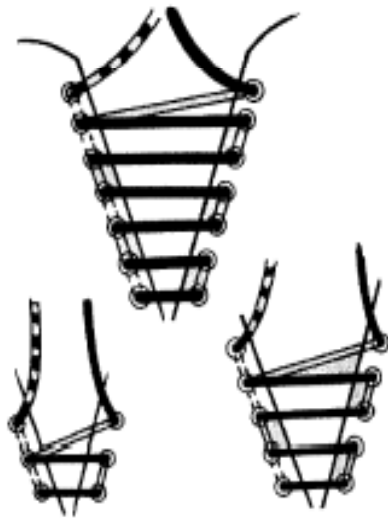
STRAIGHT ACROSS METHOD LAÇAGE TRANSVERSAL
